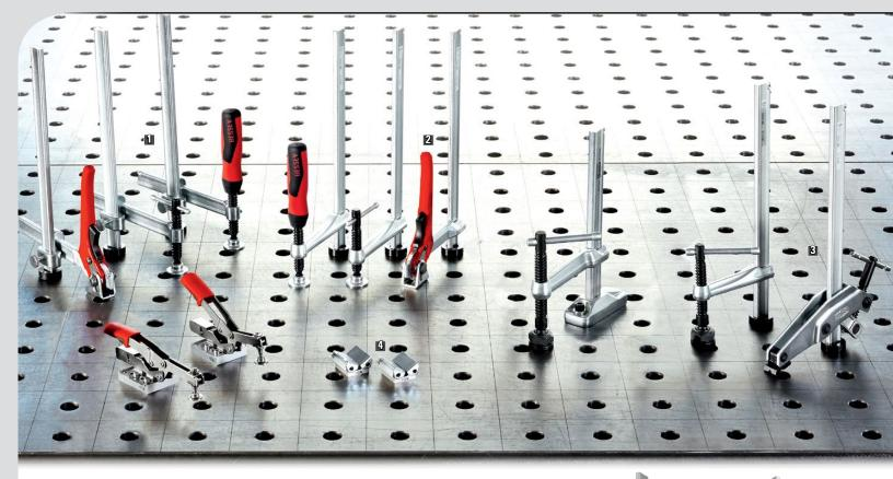
Clamping elements with 28 mm or 16 mm matrix holes. 3 handle designs for standard elements, plus variable or fixed throat depth versions. Our line-up includes a clamping element with heat-resistant pressure plate, a gripping arm variant for easy work area access, and attachments for clamping oval, round and square workpieces.
